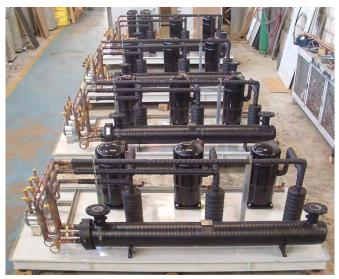
The **COOLER®** Air **Cooled Packaged Liquid Chillers** is a packaged unit completely factory assembled on a stiff steel structure with panels made from heavy gauge zinc galvanized or zinc or primered sheets with a baked fine enamel finish, making them weather resistant and suitable for outdoor installations. All piping and electrical wiring are ready for external field connection.
